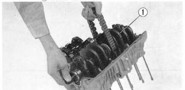
Fig. 3-65 ① Crankshaft
