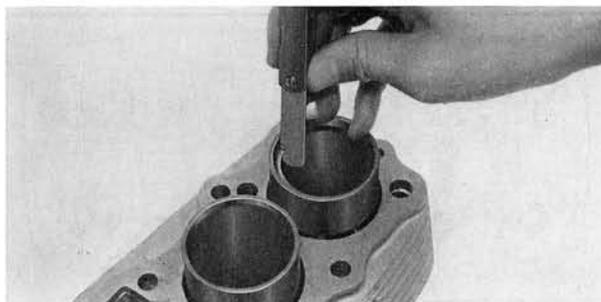
Fig. 3-16 Checking piston ring end gap
