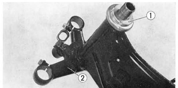
Fig. 4-44 ① Steering head top thread
