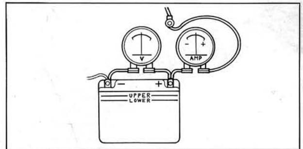
Fig. 5-11 Charging test
