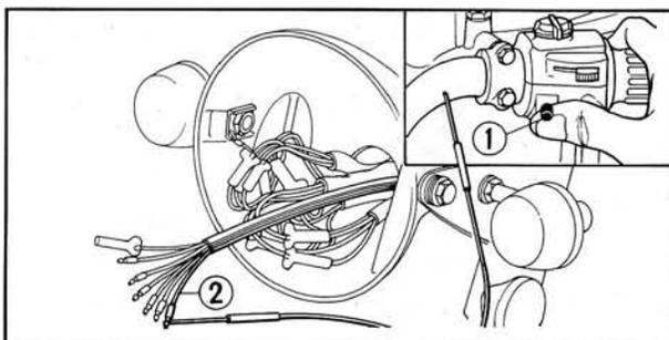
Fig. 5-41 ① Starter switch
