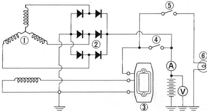
Fig. 5-12 Charging test circuit
