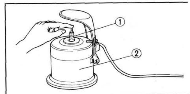
Fig. 5-6 ① Spark plug ② Plug cleaner
