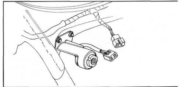
Fig. 5-34 Checking main switch
