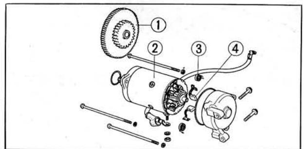
Fig. 5-24 ① Starting motor reduction gear
