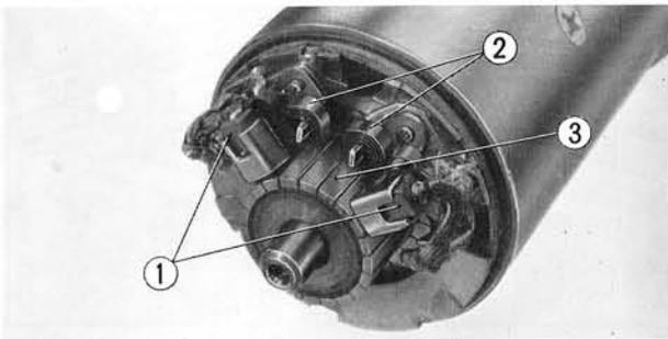
Fig. 5-25 ① Carbon brushes ② Brush springs ③ Commutator
