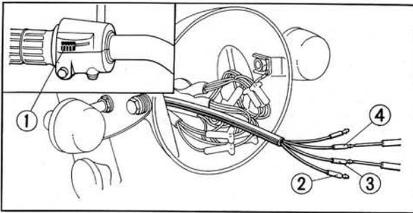
Fig. 5-38 ① Turn signal control switch
