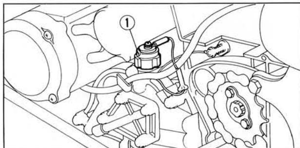
Fig. 5-43 ① Oil pressure control switch
