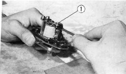
0 ① Checking point gap with a feeler gauge
