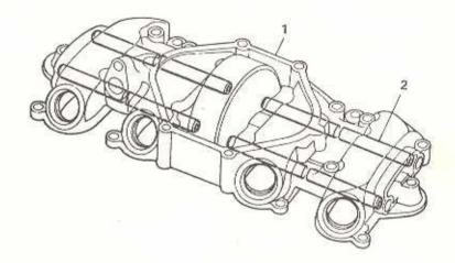
New, improved parts design prevents rocker arm shaft rotation and extends the service life of the cylinder head cover.
