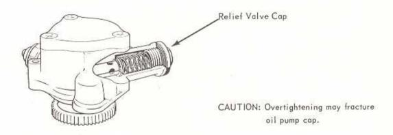
Correct oil pressure valve cap tightening torque is 7.2-10 ft.lbs. (1.0-1.4 Kg.m.).
