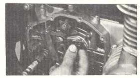
4. Remove shift drum stopper cam and the one protruding gearshift drum pin. Discard screw and pin.
