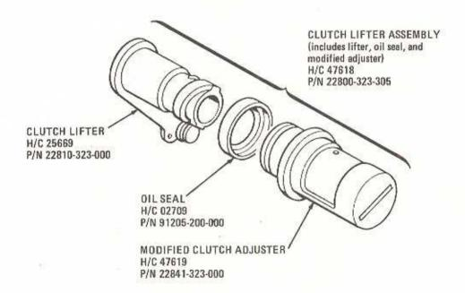
If the clutch does not work well because it is excessively worn, replace with the new clutch lifter assembly shown above.
