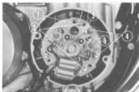
① Contact breaker base plate ② Base plate locking screws ③ Contact breaker right base plate ④ Right base plate locking screw ⑤ 1,3 cylinder breaker points
