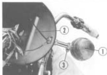
① L front turn light ② Turn light cord ③ 6x28 bolt (chrome), 6mm washer, 6mm nut
