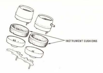
Instrument inaccuracy or needle fluctuation is frequently caused by vibration transmitted through the instrument mounting and does not necessarily involve any defect in the instrument itself.
