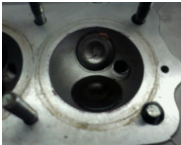
CB550 Combustion Chamber
