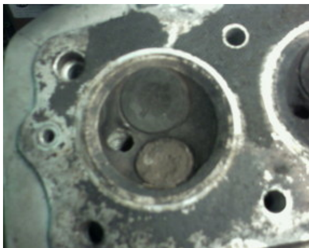
CB550 Combustion Chamber
