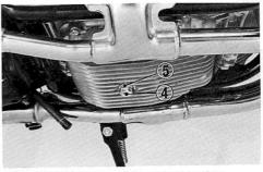
(4) Oil drain plug (5) Sealing washer
