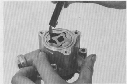
Measure the pump body clearance.
