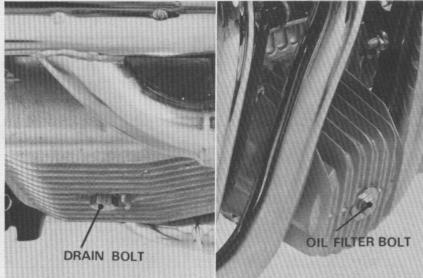
Check that the sealing washer on the drain plug and the O-rings on the oil filter bolt and oil filter are in good condition.
