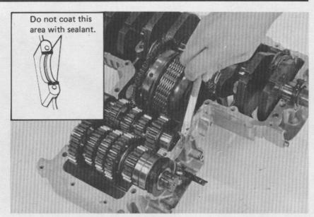
Make sure the transmission bearings and oil seal are properly seated in the upper crankcase.
