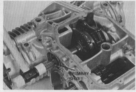
Install the bearing stopper plate.
