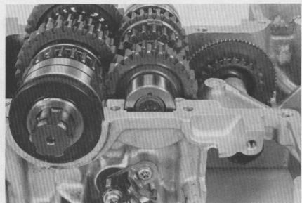
Position the primary chain and damper assembly in the crankcase.
