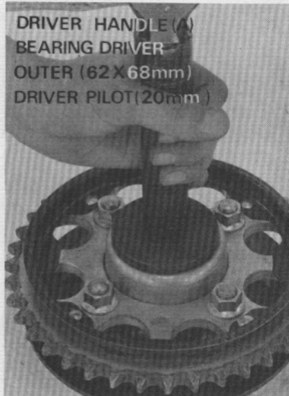
DRIVER HANDLE (A) BEARING DRIVER ATTACHMENT 07946-3290000 DRIVER PILOT (25mm)
