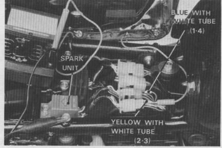
Ground each corresponding terminal (1.4: blue with white tube wire terminal, 2.3: yellow with white tube wire terminal) of the 4-pole coupler intermittently.
