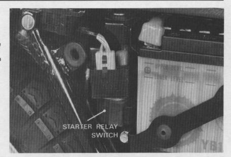
Connect an ohmmeter to the starter relay switch terminals.
