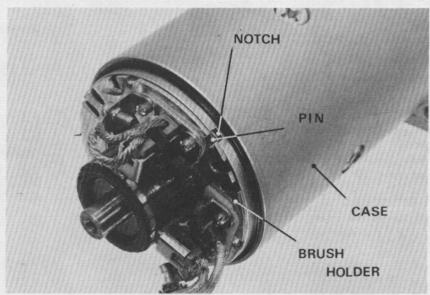
Install the rear cover aligning its slot with the brush holder pin.
