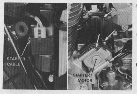
Remove the starter motor cover and starter motor.
