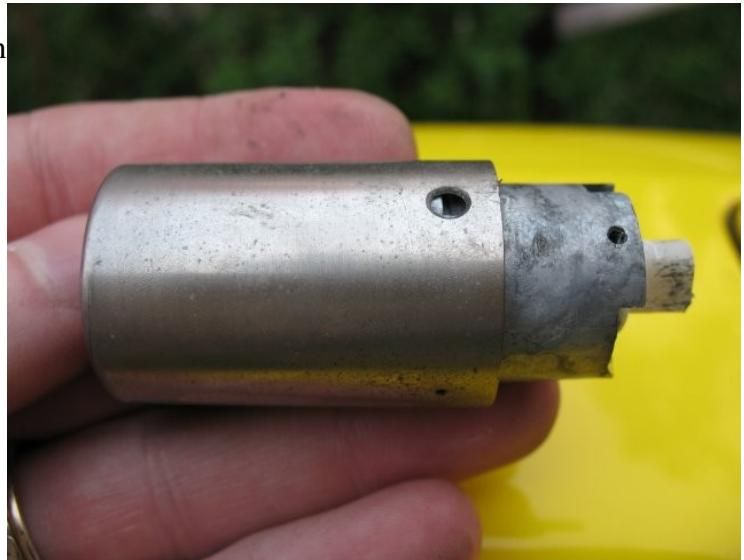
Remove the cover and take the lock to anyplace that cuts keys and tell them you want a blank that fits. Buy a couple. I wound up with an ILCO blank number X181 HD90. It's a car key so it's a bit long, but it works.
