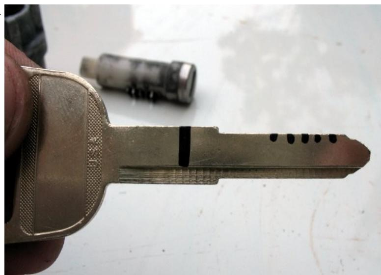
Now insert the key and notice how far the first pin protrudes. Take the Dremel and cut a notch in the bottom side of the key the depth that the pin protruded. Re-insert the key and check that the pin is now flush with the surface of the cylinder. Repeat the process for the other four pins.
