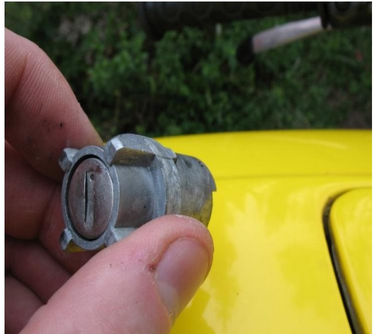
Once you're back home and fortified with a good beer (I prefer my own homebrew) start removing the core. Apply light pressure to the back of the core, insert a thin screwdriver, flat piece of metal, or chunk of zip tie you found on the floor into the keyway and depress the pins front to back to remove the cylinder.
