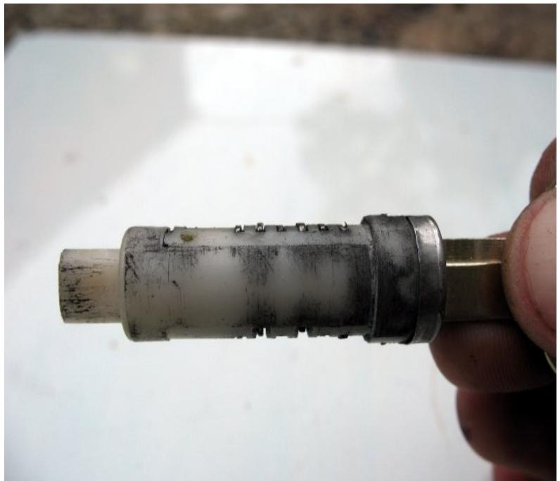
Now install the cylinder, and insert the core on the bike (line up the indicator dot), install cover, set screw and idiot light cover.
