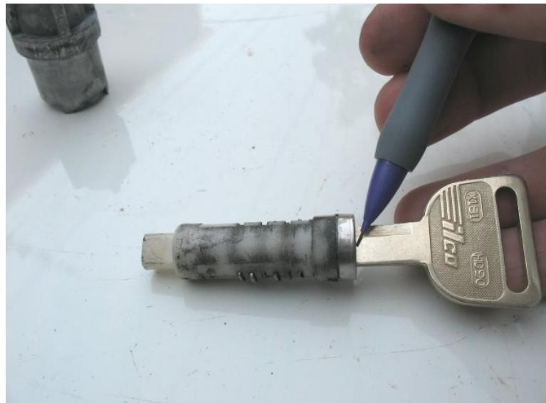
Now, place the key up against the pins and align the mark with the top of the cylinder.
