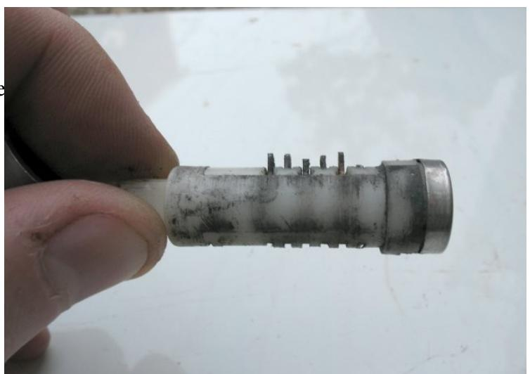
Insert your key blank fully and draw a line with a sharpie marker at the top of the cylinder.
