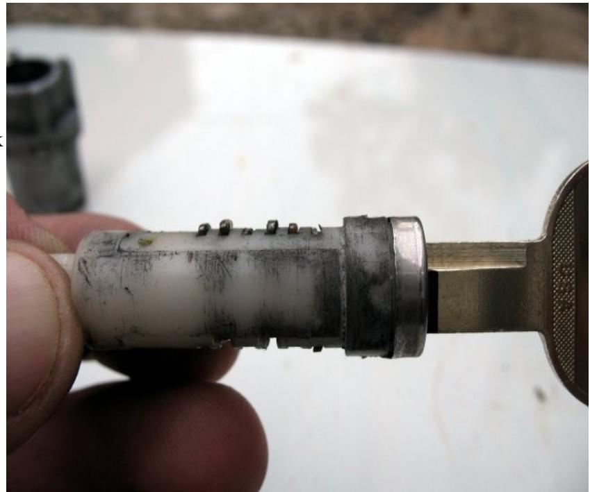
Insert the key in the keyway, reassemble the lock and check that it rotates freely. Now cut identical notches on the other side of the key and test fit that side as well.
