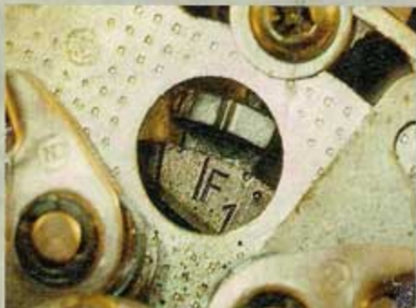
F-mark is for strobe check firing at idle
