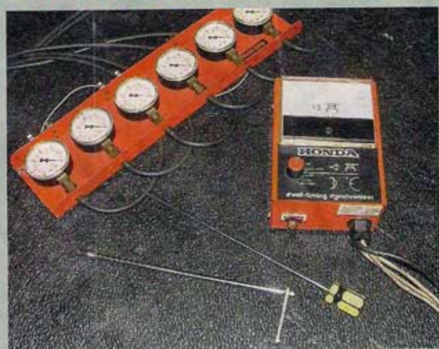
John Wyatt's Davida vacuum gauges for synchronising carburettors; his factory Honda dwell meter for ignition points setting; and a carb adjusting tool set with spanner and long screwdriver
